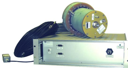
AT-7000 for Brake Temperature Testing
