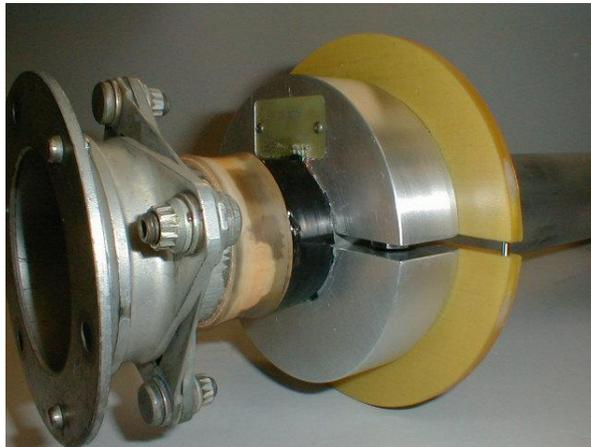
The picture shows an aluminum clamp collar securing the Transmitter’s single channel electronics module to the high speed shaft. To couple power to the rotating transmitter (and to retrieve the digital data stream coming back to the Receiver), a glass laminate assembly (larger diameter yellow disks) is interconnected to the aluminum collar. A simple pickup loop (not shown) was used to provide the power and data connection to a Receiver located 24 feet away.
