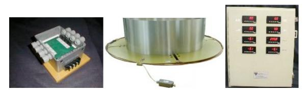
The above left picture shows the rotating Transmitter for the 8 RTD's (cover removed to show connections for the RTD's), the induction power/data coils (during testing in Schenectady) in the center, and the Receiver (digital to analog output device) on the right. The Receiver is equipped with optional panel meters providing y=mx+b unit translation (analog voltage to scaled temperature outputs).
